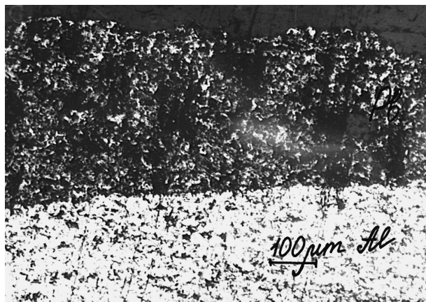
Fig. 2. Cross-section ( \times 100 ) of lead-film electrode before cycling.
